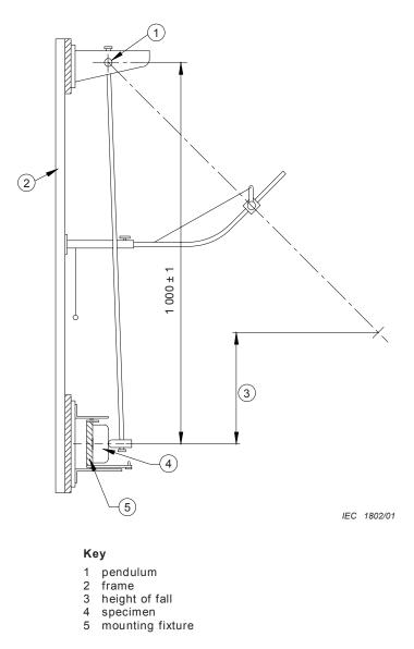
Figure 4 – Impact test apparatus
